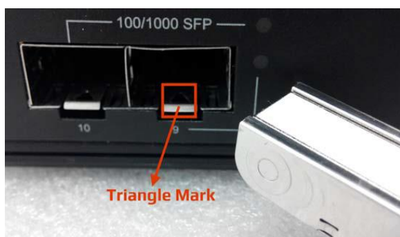
Figure 2.6 - Transceiver to the SFP Slot
