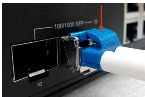
Figure 2.9 - Remove LC Connector
