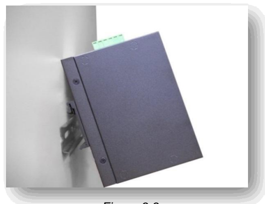
Stable the Switch on DIN-Rail
