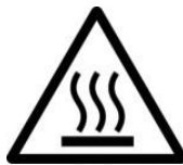
Figure 1.2 - Hot Surface Warning Label
