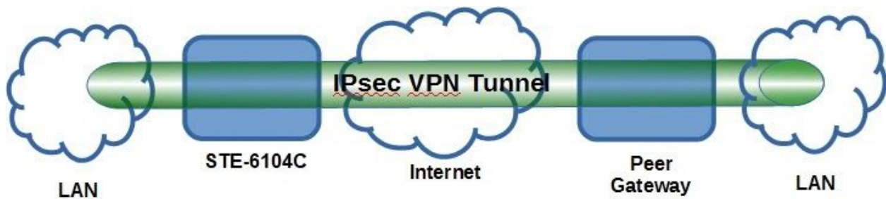
Figure 3.51 - IPsec VPN Tunnel with Network-to-Network Topology
