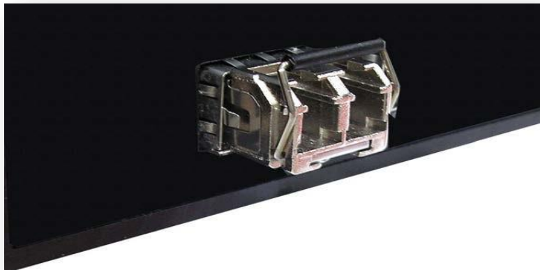
Figure 2.10 Transceiver Inserted
