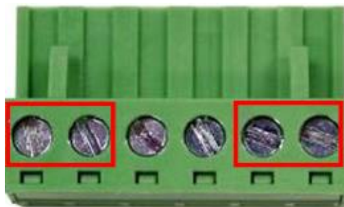
Figure 2.15 Power Terminal Block
