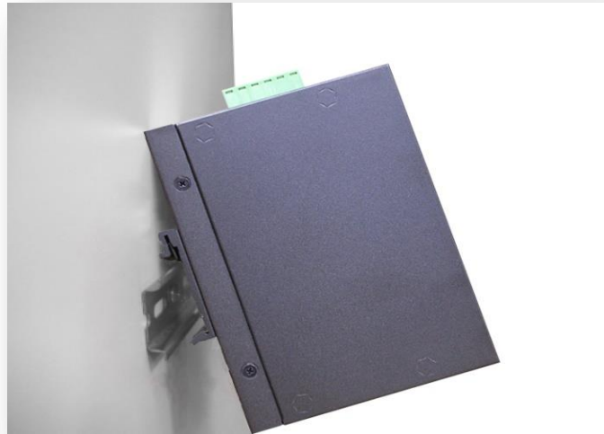
Figure 3.2 Insert the Switch on the DIN-Rail
