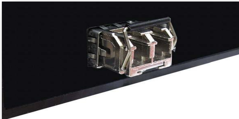
Figure 2.10 Transceiver Inserted
