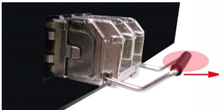
Figure 2.13 Pull Out from the SFP Module
