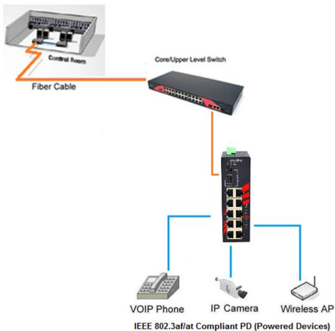
Figure 5.1 Industrial Ethernet Switch Application Reference
