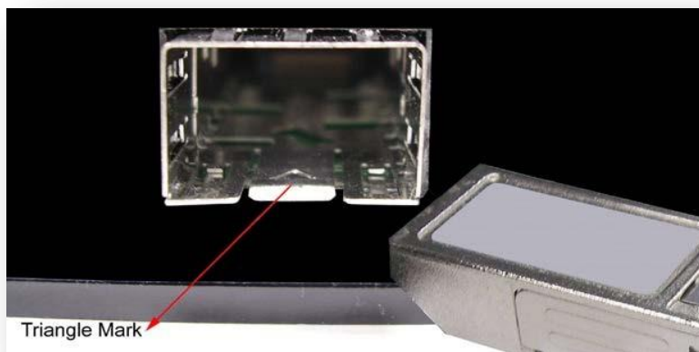
Figure 2.9 Transceiver to the SFP Module
