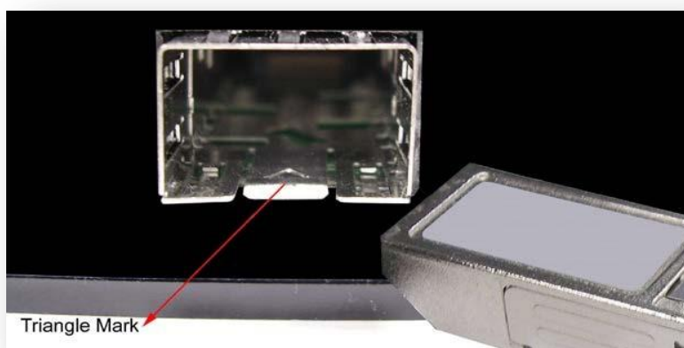
Figure 2.9 Transceiver to the SFP Module
