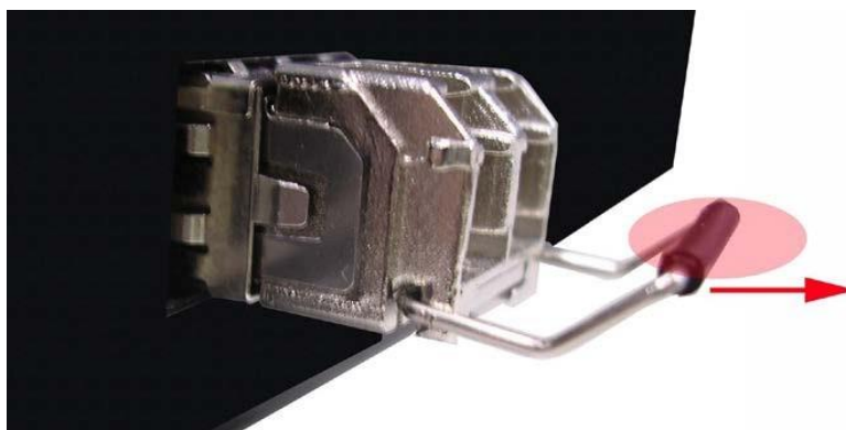
Figure 2.13 Pull Out from the SFP Module
