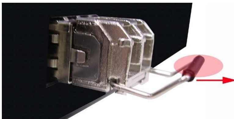
Figure 2.10 Pull Out from the SFP Module
