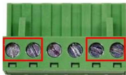
Figure 2.7 Power Terminal Block
